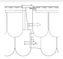
Slide the next panel into position: the top half of the panel, except the nail hem, slides under. The bottom half slides over the previous panel.
