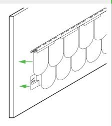
A solid nailable sheathing, such as plywood or OSB and a water resistive barrier (WRB) is necessary for a proper and secure installation.
