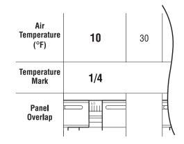
Let panels acclimate to the air temperature. Air temperature should be checked **ONLY** when installing the first course of each new wall to determine the amount of panel overlap.
