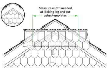
the gable. Temporarily fasten through the center hole. Continue temporarily installing full panels toward right side of the gable to establish where to cut the right end of the first panel.
