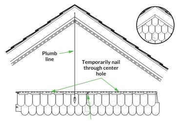
The top piece should be centered at the peak of the gable for proper appearance. For symmetrical appearance at the peak, position and lock a full panel in the first course with Half-Rounds at the center of
