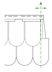
Panels must always be installed from right to left. Cut the first panel in the first course at "A". Allow 1/4" gap at all corner posts, J-Channel, or other stops.
