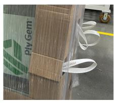
Modular packaging: Frame pieces and door panels are packed and shipped together with the hardware kit and match the bill of materials for a customer's order.
